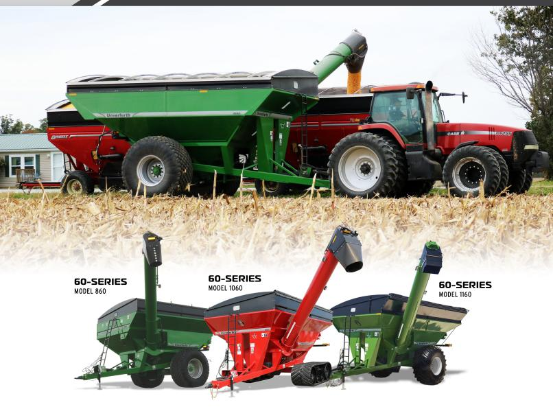
If you need additional unloading auger side-reach and height, look to the Unverferth 60-Series lineup of corner-auger grain carts. The side-folding design allows the upper auger to be longer, so you can reach over ditches and clear the tallest trucks. Tank capacities range from 630 to 1,100 bushels and unloading speeds up to 500 bushels per minute to get you back to the combine faster.
